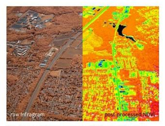
Combine an infragram camera with Public Lab's open source Balloon Mapping Kit for aerial infrared plant analysis!
