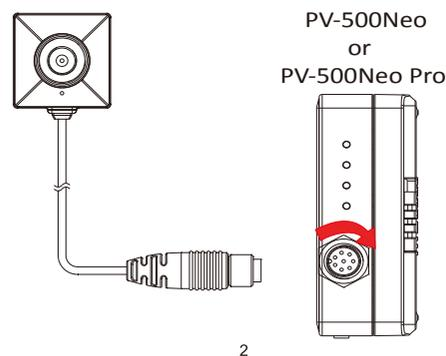
To connect the camera to the DVR, fully plug the camera's connector end into the **Camera In** port on the DVR, then lock the connector firmly by rotating it to the direction of the red arrow.
