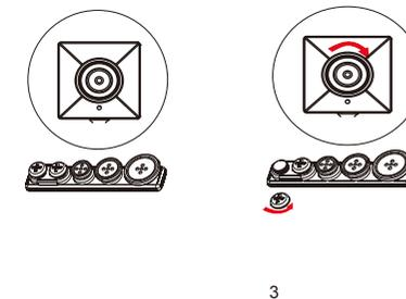
1. Unscrew the preferred lens cover cap at counterclockwise direction to remove it from the set.
