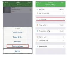
4. Select the router Wi-Fi and input the password, the camera will then connect to the router, enabling you to view the live feed while outside of your home network.
